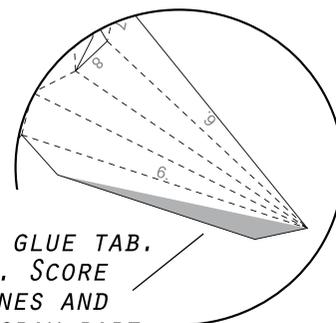
THIS IS A SPECIAL GLUE TAB. CUT OUT THE SHAPE. SCORE ALL THE DASHED LINES AND THEN CUT OFF THE GRAY PART.
